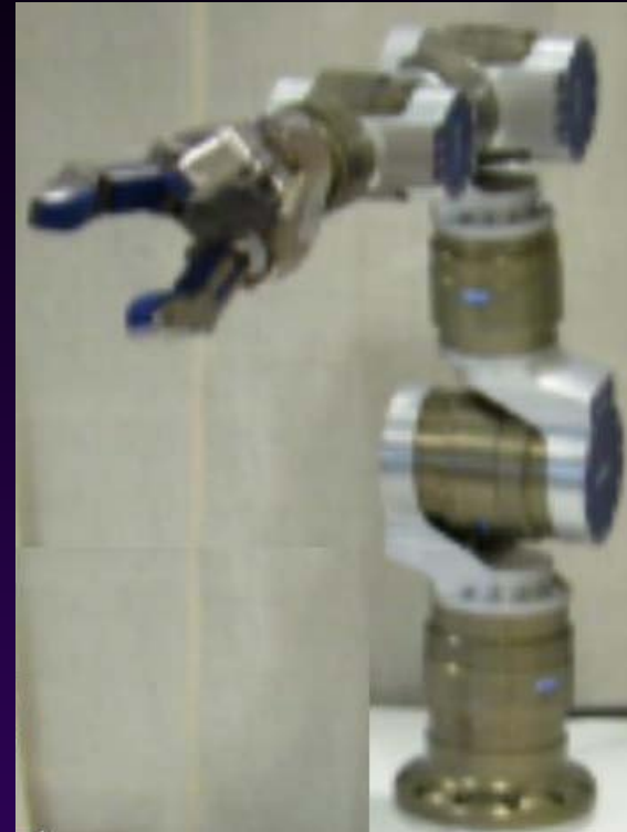
Schunk 7DOF arm with 3-fingered gripper
