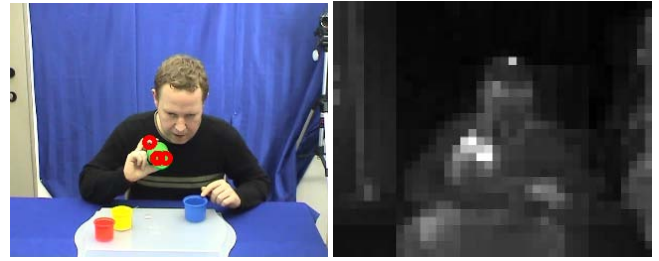
(a) input image, in which attended locations denoted by circles (b) saliency map (sum of (c)-(g))
