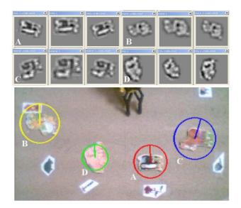
Figure 3. Vision processing. Above: A. – D. Three templates each for the Dog, Duck, Horse and Pig objects at three different orientations. Below, encompassing circles indicate template recognition for the four different objects near different fixed landmarks, as seen from the camera over the robot workspace
